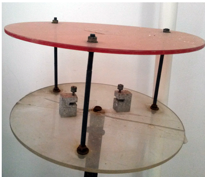
Fig. 1 Image of the Durham trap which was exposed at the monitoring Site 1 (Tab. 1). It is kept now set-up in the Aerobiological Laboratory of VNMU, Ukraine.
